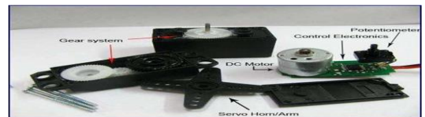
Fig.4.6: Components of servo motor [7] .
